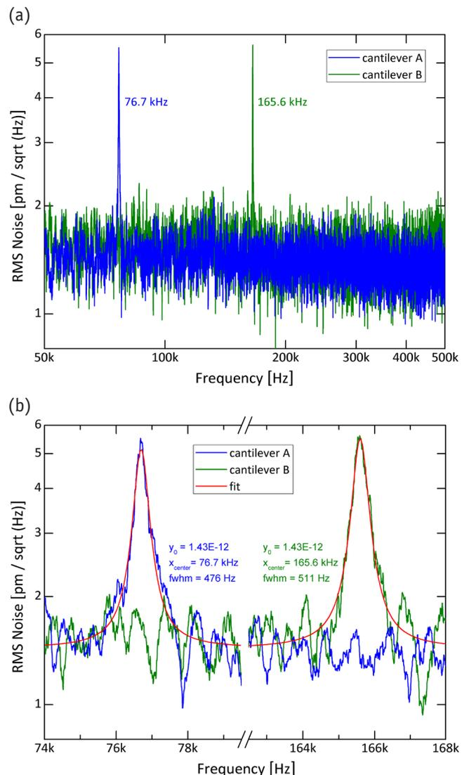
**Figure 2:** The figures (a) and (b) show the FFT analysis of the two different cantilevers under investigation. The resonant frequencies of the cantilevers can be seen at 76.7 kHz (thin cantilever A) and 165.6 kHz (thick cantilever B).
