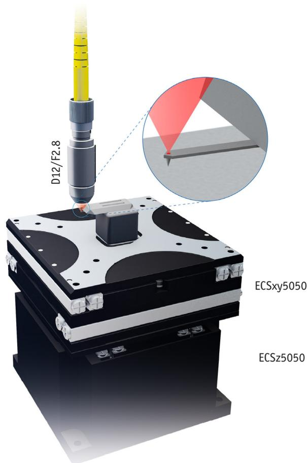
**Figure 1:** A stack of three attocube x-, y-, and z-positioners was used to align the D12/F2.8 sensor head onto the micro-cantilever. The distance between the objective and the cantilever was about 2.8 mm.
