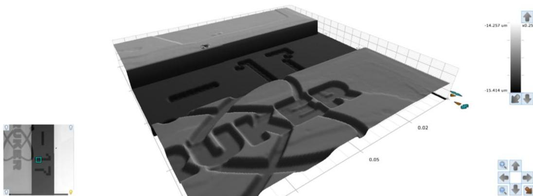
*3D optical microscopes provide detailed surface topography data*
