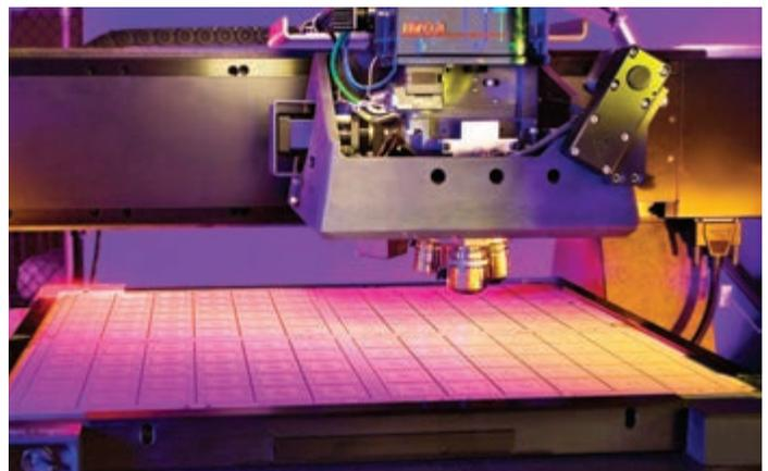
*A 3D optical microscope measures an MCM panel.*
