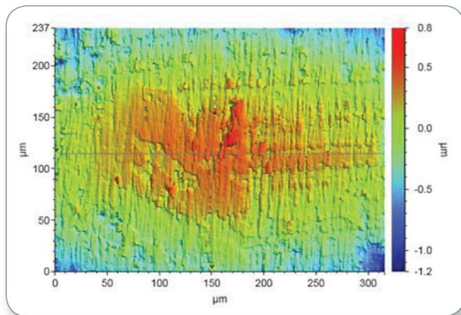
Figure 3. Surface topograph of the piston ring before performing the engine test, obtained with a Bruker ContourGT interferometer.
