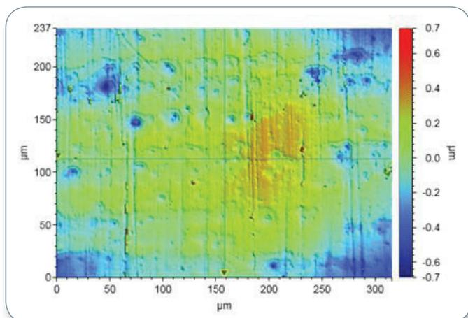
Figure 4. Surface topograph of the piston ring after performing the engine test, obtained with a Bruker ContourGT interferometer.
