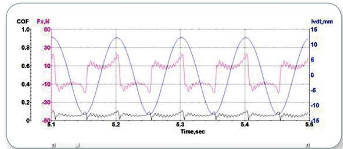
Figure 1. Plot of friction force ( $F_x$ ), stroke position (lvdt), and coefficient of friction (COF) as a function of time for a test of piston ring on a cylinder liner segment with a normal load of 200N in lubricated condition.
