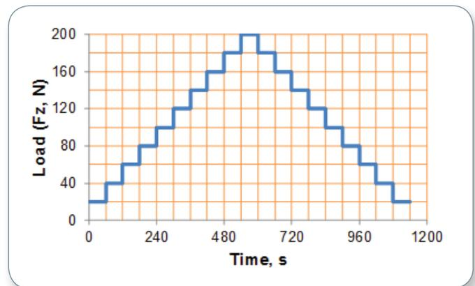
Figure 2. Normal load profile ( $F_z$ ) as a function of time for an engine test.
